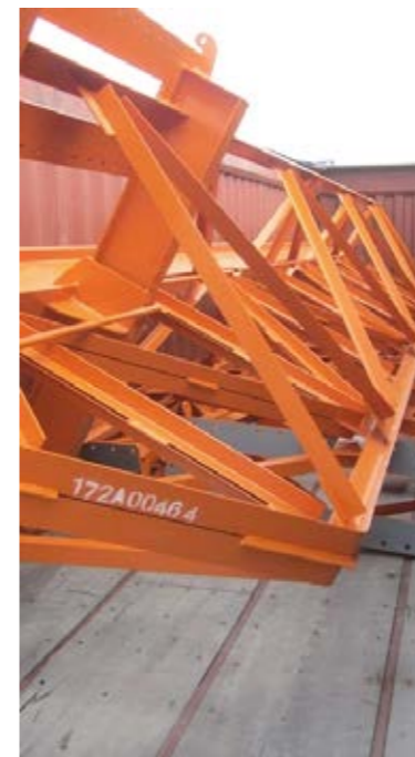
1set 10t Trussed Single Girder Gantry Crane Exported to Philippines
